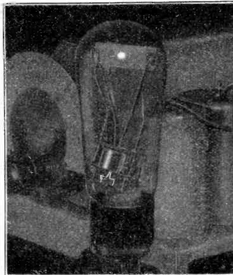
The "Tunograph" indicator, showing the light spot on the screen. As the tuning is varied to bring the set into resonance with the signal, the light spot moves to the right.
